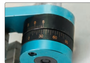
Calibration w/ Vernier
