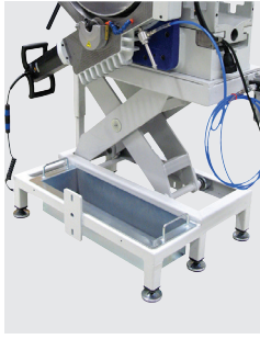
Including a height-adjustable and robust lifting bench with a container for swarf collection
