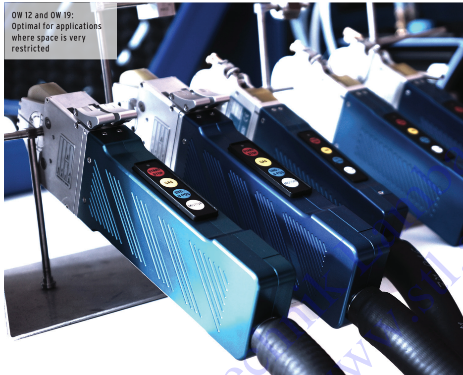
The 3-part clamping mechanism ensures that the head can be clamped even in the most confined spaces
