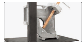
Machined Outside Faces for upright joint.
